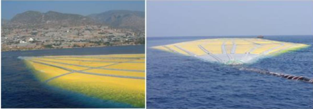
Figure 3. Medusa bags floating on the Mediterranean Sea, carrying fresh water from Turkey. Source: (Yıldız and Çakmak 2014).
