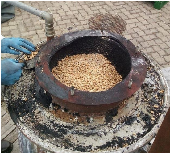
Figure 11. Downdraft gasifier with wood pellets as feed
